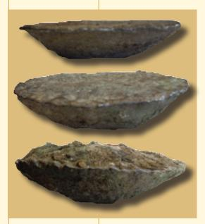
Above, from top to bottom: Silver alloy ingot, 17–18cm diameter, 5.5 kg, 76% silver, 13% gold; Silver alloy ingot, 21–23cm diameter, 11 kg, 82% silver, 3% gold; Copper alloy ingot, 32–35cm diameter, 25 kg, metal content not analysed.
